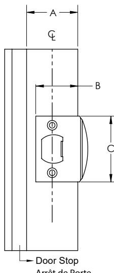
Dimension B & C should be used as reference only. Due to tolerances as reference only. Due to tolerances actual door jamb prep dimensions will vary. Using the strike plate outline edges and locate screw holes on strike with center line on jamb.
